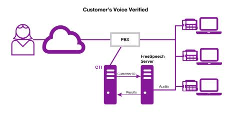
FreeSpeech's main component is called the Processing Server. It hosts the speaker verification engines, which perform algorithmic processing, control client services, and acquire audio through API calls.
